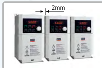
Side-by-side Installation (2mm between drives)
