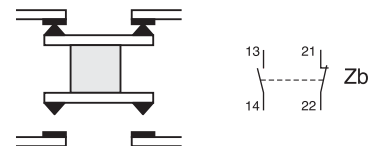
The 2 moving contacts are electrically separated
