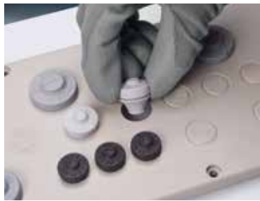
Place the grommet on the hole and pull it firmly to its place.
