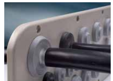
(Front side) Pull the cable or tube back for some 20 mm to lock it.
