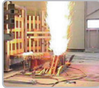
Short-Circuit Test / ACB Breaker Test
