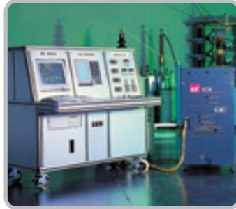
Characteristics Test / VCB Characteristics Test
