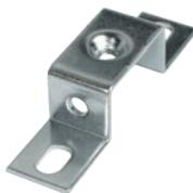
It is possible to place DIN rails on the flat brackets horizontally to the wall. All brackets have an opening with metric thread M6 piece for easy and convenient connection to the DIN rail. DIN rail brackets are made of steel surfaced by zinc.
