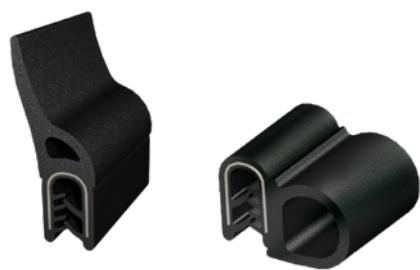
Self-gripping sealing profile made with a black PVC carrier with sealing lip or sealing tube from EPDM. Integrated steel strip core. Other colors are available on request.
