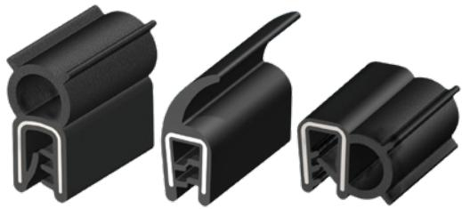
Self-gripping sealing profile with a black EPDM rubber carrier and a sealing lip and / or sealing tube from sponge-rubber. Integrated steel strip core or steel wire core.
